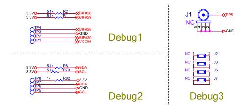
Figure 7-1 Debug Ports
