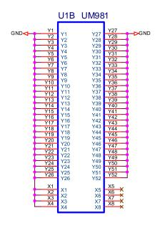
Figure 6-3 Pads (Y1-Y52) and Socket Mounting Holes (X1-X8)
