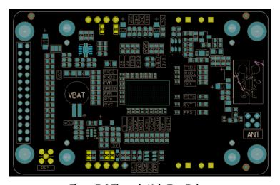
Figure 7-2 Through-Hole Test Points
