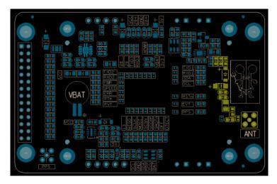
Figure 4-4 Antenna Feed Circuit on the Bottom of the Evaluation Board
