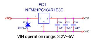
Figure 3-1 Power Filter Circuit
