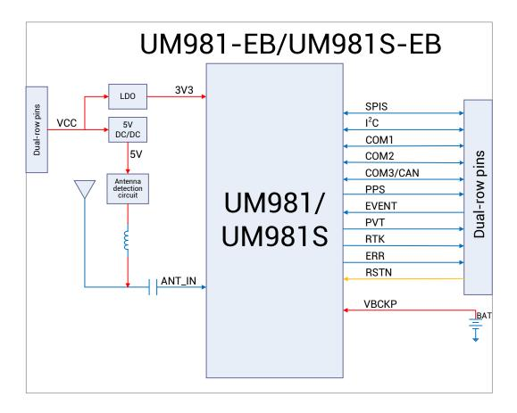
Figure 1-1 Block Diagram
