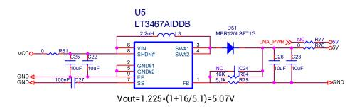
Figure 3-4 5V DC/DC Boost Circuit
