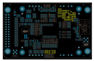
Figure 4-2 Antenna Detection Circuit on the Bottom of the Evaluation Board
