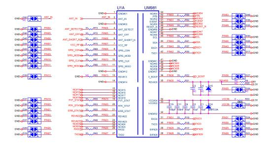
Figure 6-1 UM981 Series Module's Peripheral Design
