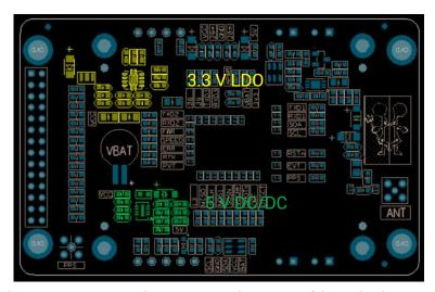
Figure 3-2 3.3 V LDO and 5 V DC/DC on the Bottom of the Evaluation Board
