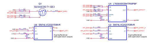
Figure 4-1 Antenna Detection Circuit
